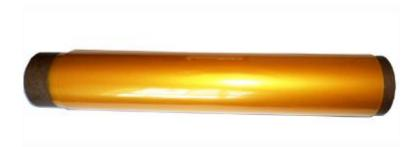
In addition to the very good performance of high and low temperature resistance, electricity insulativity, radiation and etching resistance, it also has very excellent performance of corona resistance and thermal conductivity. The corona polyimide film applies to turn-insulating, major insulation, external insulation of big coil and corona resistance protective layer of large tractive motor, conversion motor, wind driven generator, special motor etc.
