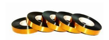
Polyimide pressure sensitive adhesive tape with silicone resin, This kind of tape is made of polyimide material with heat-resistant silicone adhesive, which shows excellent dielectric insulation properties, high heat resistant, excellent solvent resistant, mask-off gold finger contacts during wave soldering, short-term temp. 250c x 5sec, and is widely used for electrical insulation on motor, transformer, coils, PCB making and so on.
